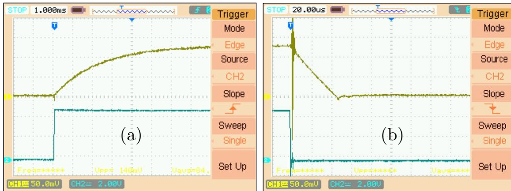
FIGURE 4.3: Magnetic quadrupole coil field response time. (a) The top trace is the current in the coils, with scale 10 mV/A. The rise time is \sim 5 ms. The bottom trace shows the rising trigger pulse for the switching circuit. (b) The top trace is the current in the coils, with scale 10mV/A. The fall time is \sim 44\mu s. The bottom trace shows the falling trigger pulse for the switching circuit.
